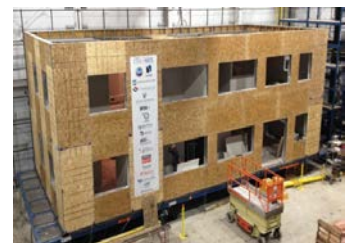
CFS NEES Building at University of Buffalo during Testing
