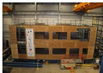
CFS NEES Building at University of Buffalo during Testing
